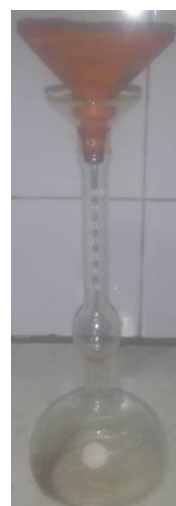
Fig. 4: Insertion of the funnel into the Le Chatelier flask
