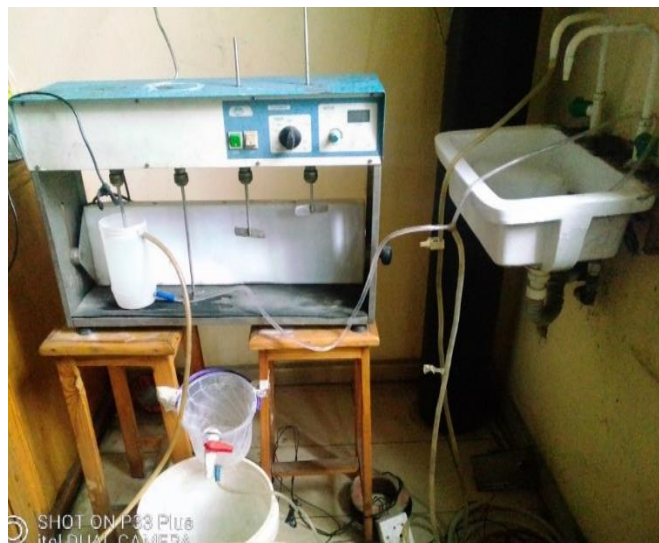
Fig. 3: Experimental setup for the desliming of the barite samples
