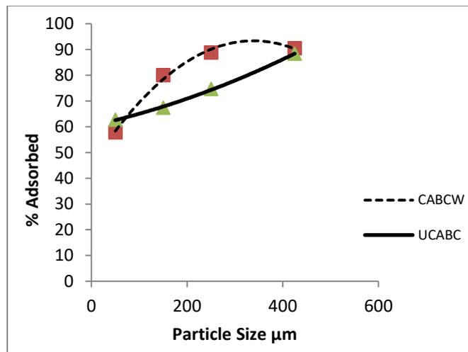
**Figure 5:** Lead removal as a function of particle size
