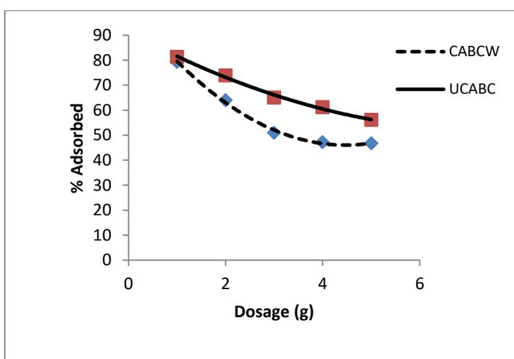
Figure 1: Lead removal as function of adsorbent dosage
