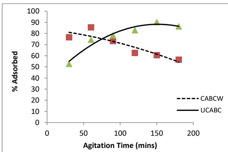
**Figure 3:** Lead removal as a function of agitation time
