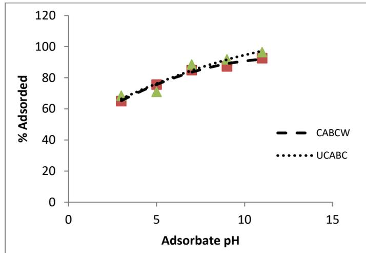
**Figure 4:** Lead removal as a function of adsorbate pH
