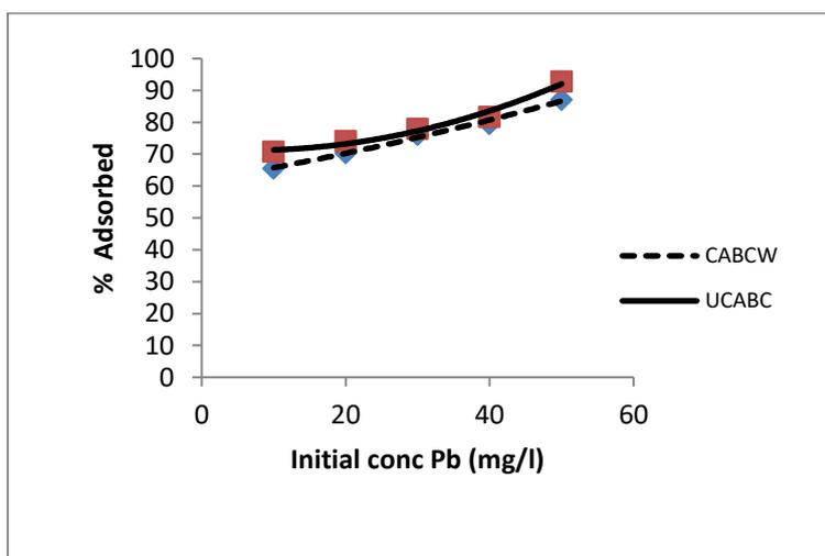
Figure 2: Lead removal as a function of initial concentration
