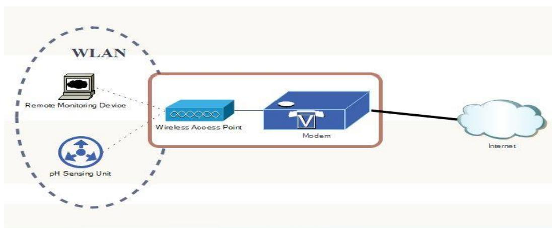
Figure 1: Network architecture of the system
