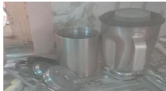
**Fig. 2:** Blending cup used to blend the cement slurry
