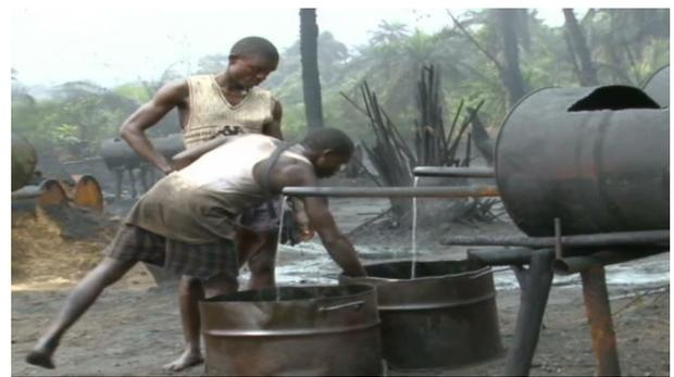
**Fig. 1:** Operators take a closer look as condensed petroleum liquids flow into products collection tanks in an illegal refinery. Source: Purefor (2010)
