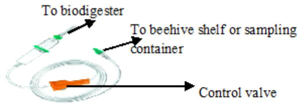
**Fig. 3:** Safety infusion set to serve both as produced gas and effluents delivery tube
