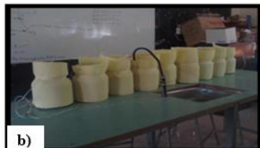
**Fig. 5:** Construction of the biodigesters by inserting (a) the ports and (b) polyurethane insulation
