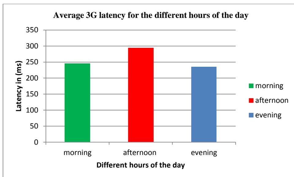
**Fig. 3:** Average 3G latency for the different hours of the day. Morning hours (8am- 11 am), afternoon hours (12noon-4pm) and evening hours (5pm-9pm) by 3G MTN network in Trans Amadi Area of Port Harcourt.
