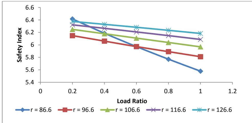
Fig. 5: Safety index against load ratio at varying radius of gyration (compression failure mode)
