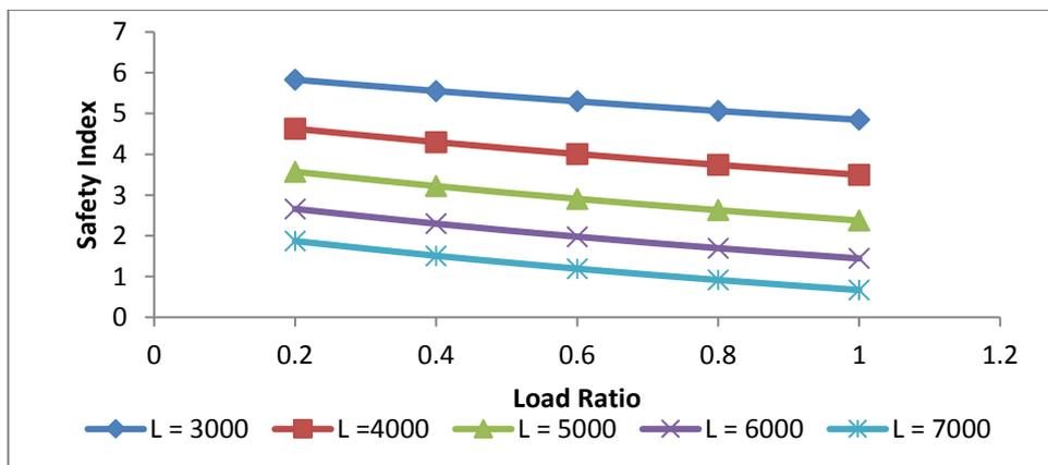
Fig. 4: Safety index against load ratio at varying length of column (bending failure mode)
