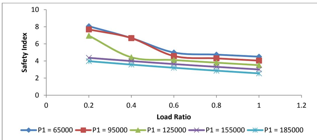
Fig. 9: Safety index against load ratio at varying axial load (compression-bending failure mode)
