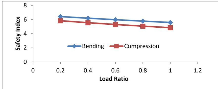
Fig. 2: Safety index against load ratio in bending and compression
