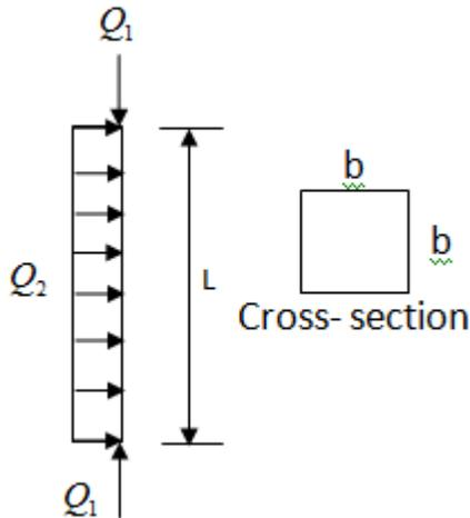
**Fig. 1:** A pin ended square timber column under compression and bending
