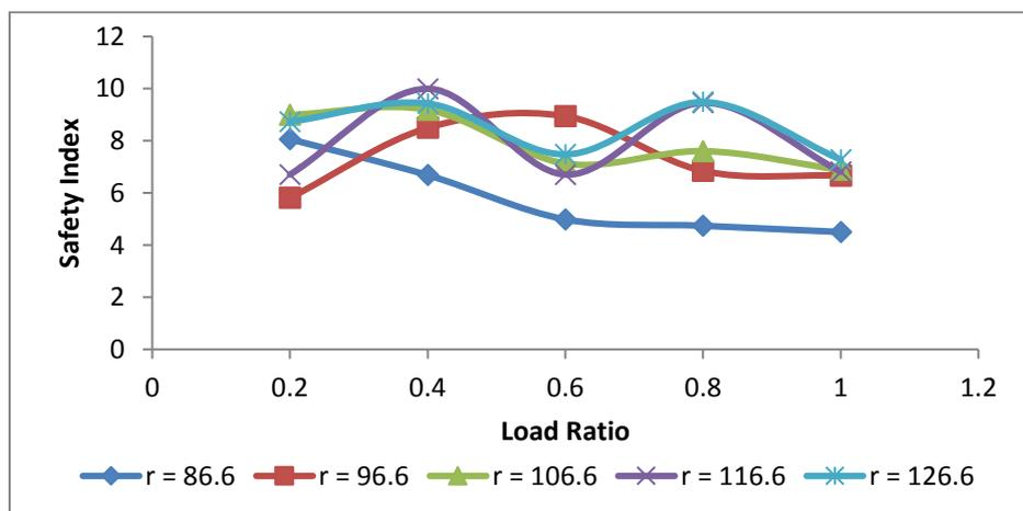
Fig. 7: Safety index against load ratio at varying radius of gyration (compression-bending failure mode)
