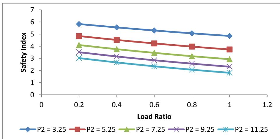
Fig. 10: Safety index against load ratio at varying lateral load (bending failure mode)
