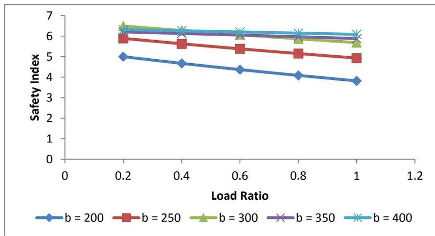
Fig. 12: Safety index against load ratio at varying column depth (compression failure mode)
