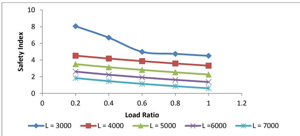
Fig. 3: Safety index against load ratio at varying length of column (compression-bending interaction failure mode)
