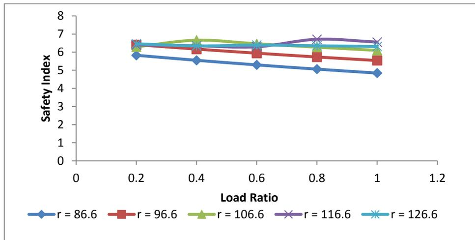
Fig. 6: Safety index against load ratio at varying radius of gyration (bending failure mode)
