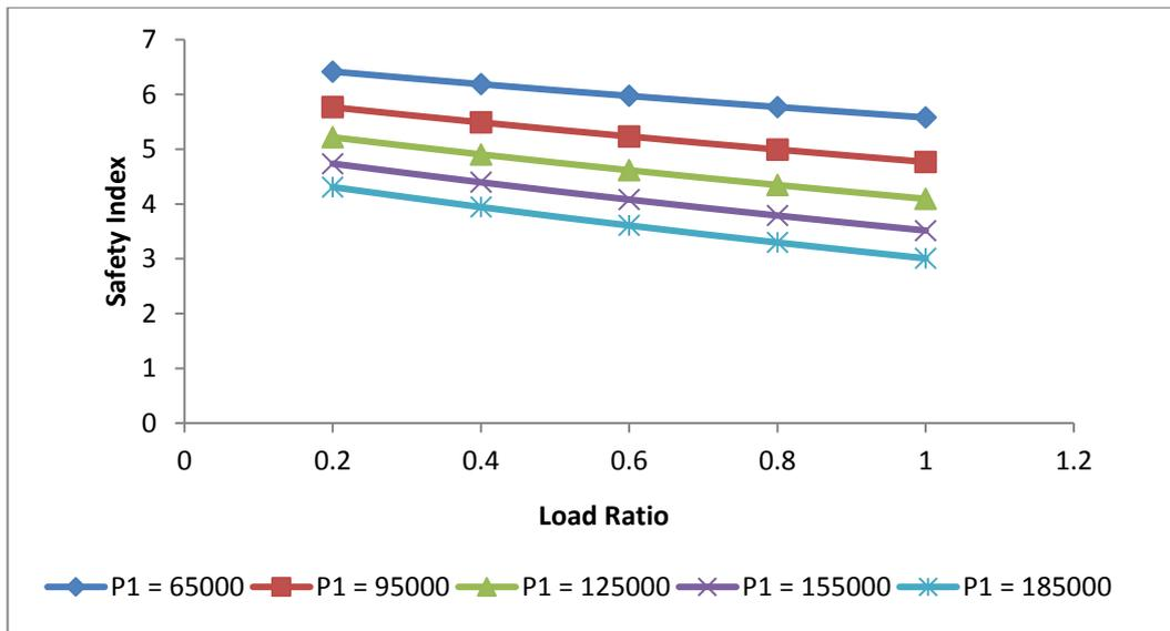
Fig. 8: Safety index against load ratio at varying axial load (compression failure mode)
