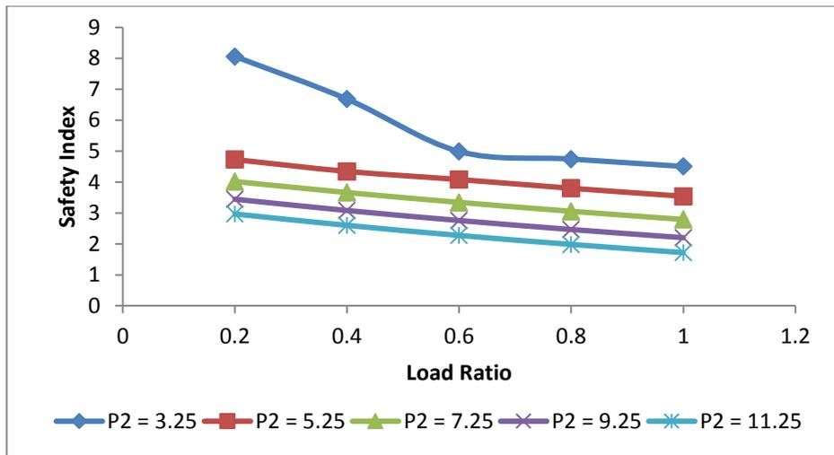
Fig. 11: Safety index against load ratio at varying lateral load (compression-bending failure mode)
