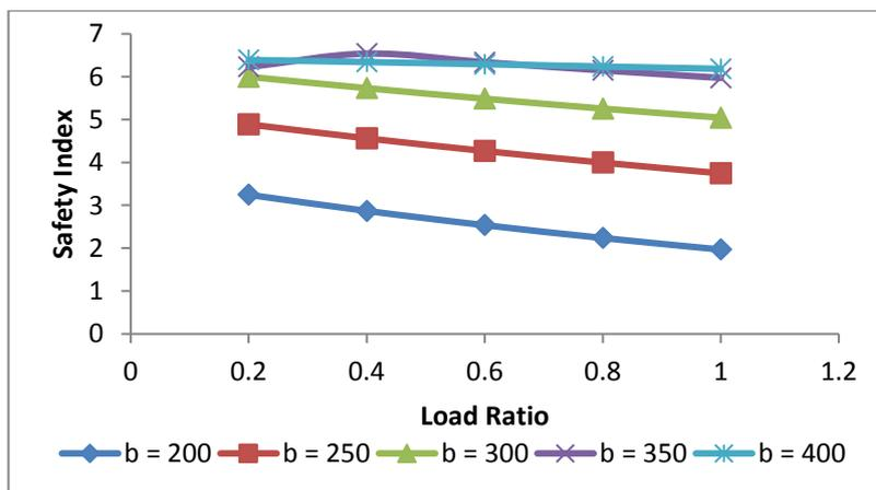
Fig. 13: Safety index against load ratio at varying column depth (bending failure mode)
