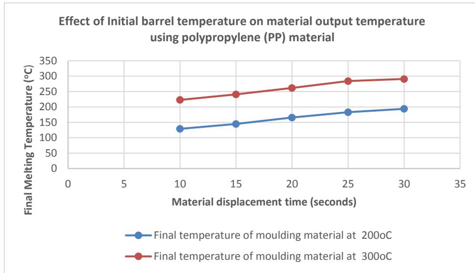
Fig. 4: Melting temperature test using polypropylene (PP) material
