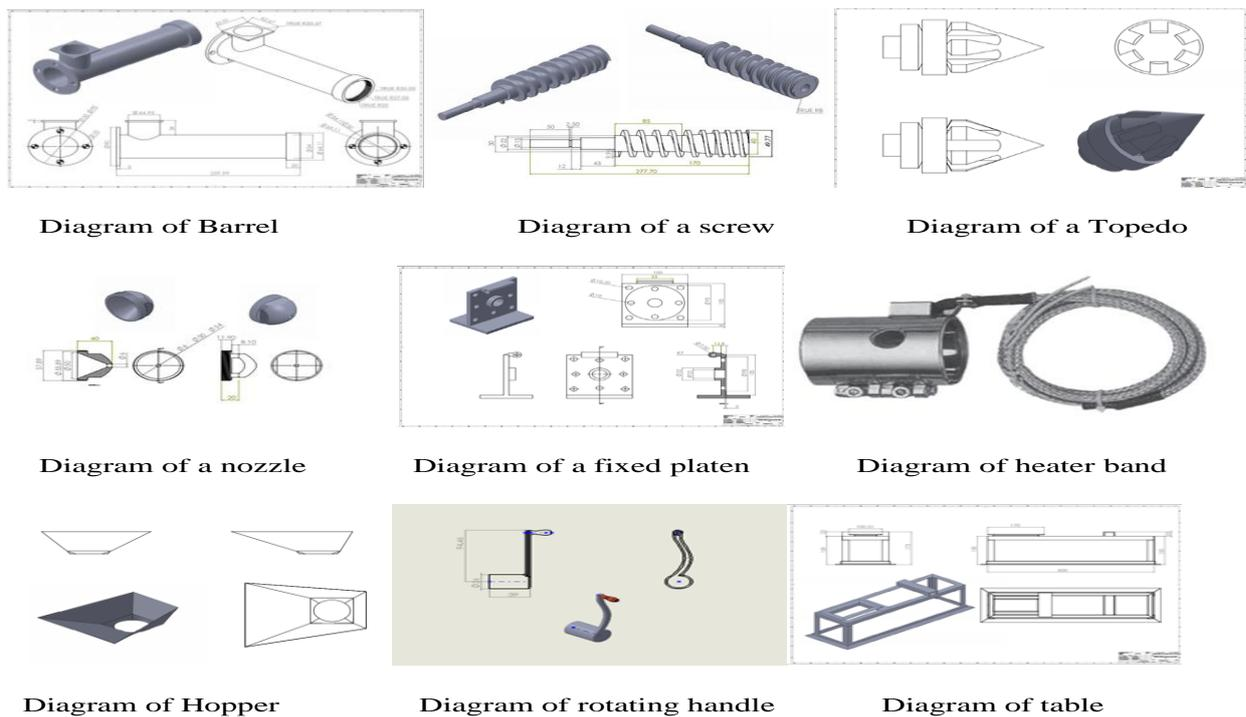
Fig. 3: Detailed drawing of injection moulding machine component
