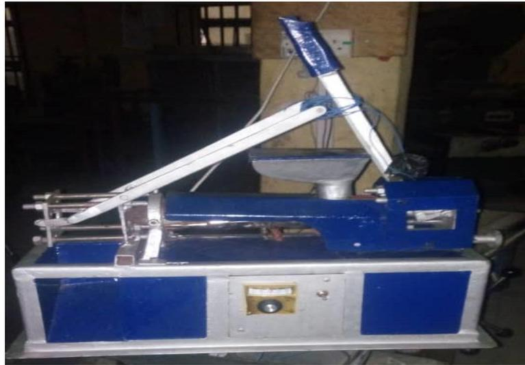
**Fig. 6:** Pictorial view of the fabricated injection machine
