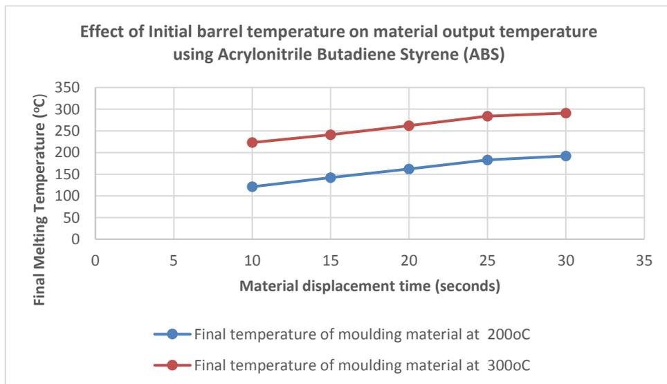
Fig. 5: Melting temperature test using Acrylonitrile Butadiene Styrene (ABS) material
