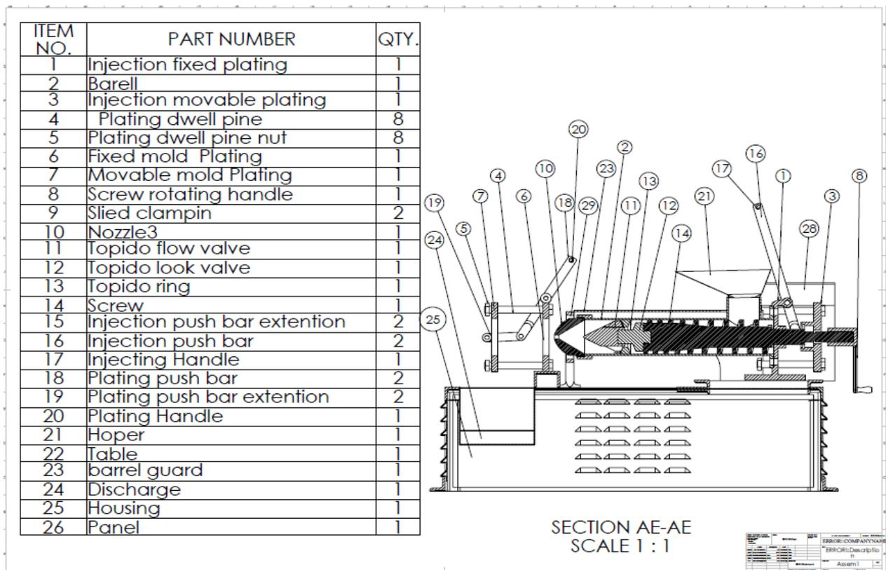
Fig. 2: Sectional view of the plastic injection machine
