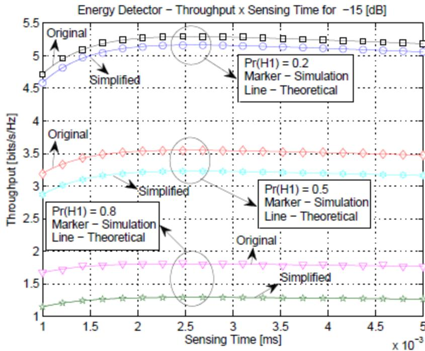
Fig. 2: Throughput vs. sensing time for SNRp = -15[dB]
