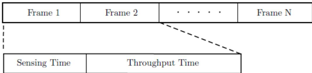
**Fig.1:** Frame structure for cognitive radio networks with periodic spectrum sensing
