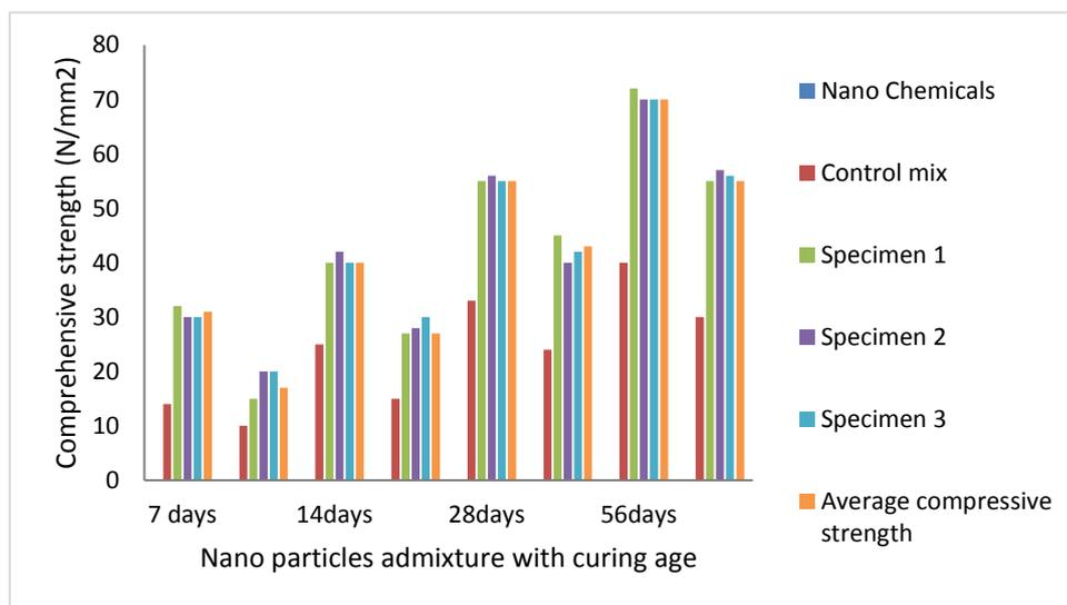
**Fig. 1:** Effect of curing age on the compressive strength of interlocking blocks
