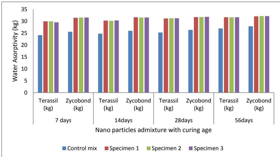
**Fig. 2:** Effect of different percentage combination of nano particles on water absorptivity of interlocking paving stones
