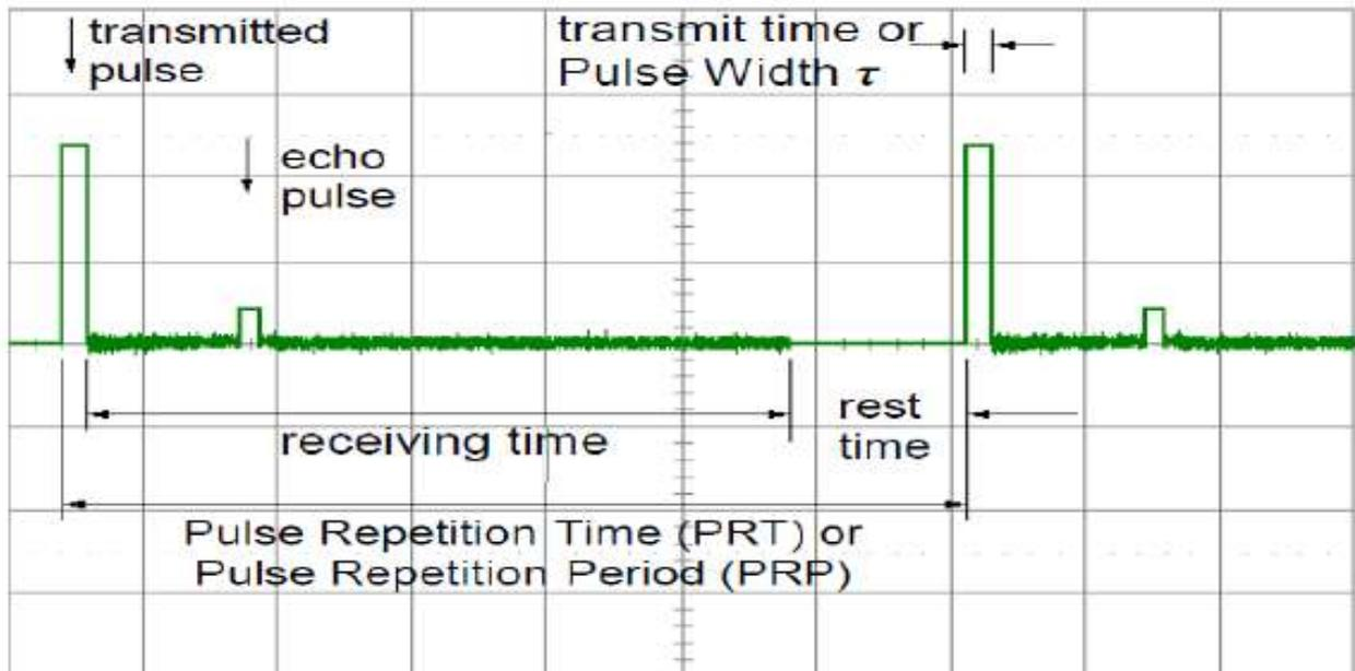
Fig. 1: Transmitted and received pulse
