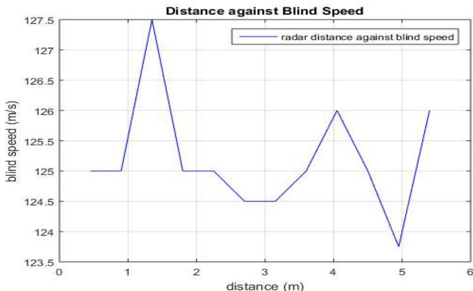
Fig. 8: Graph of radar blind speed against distance
