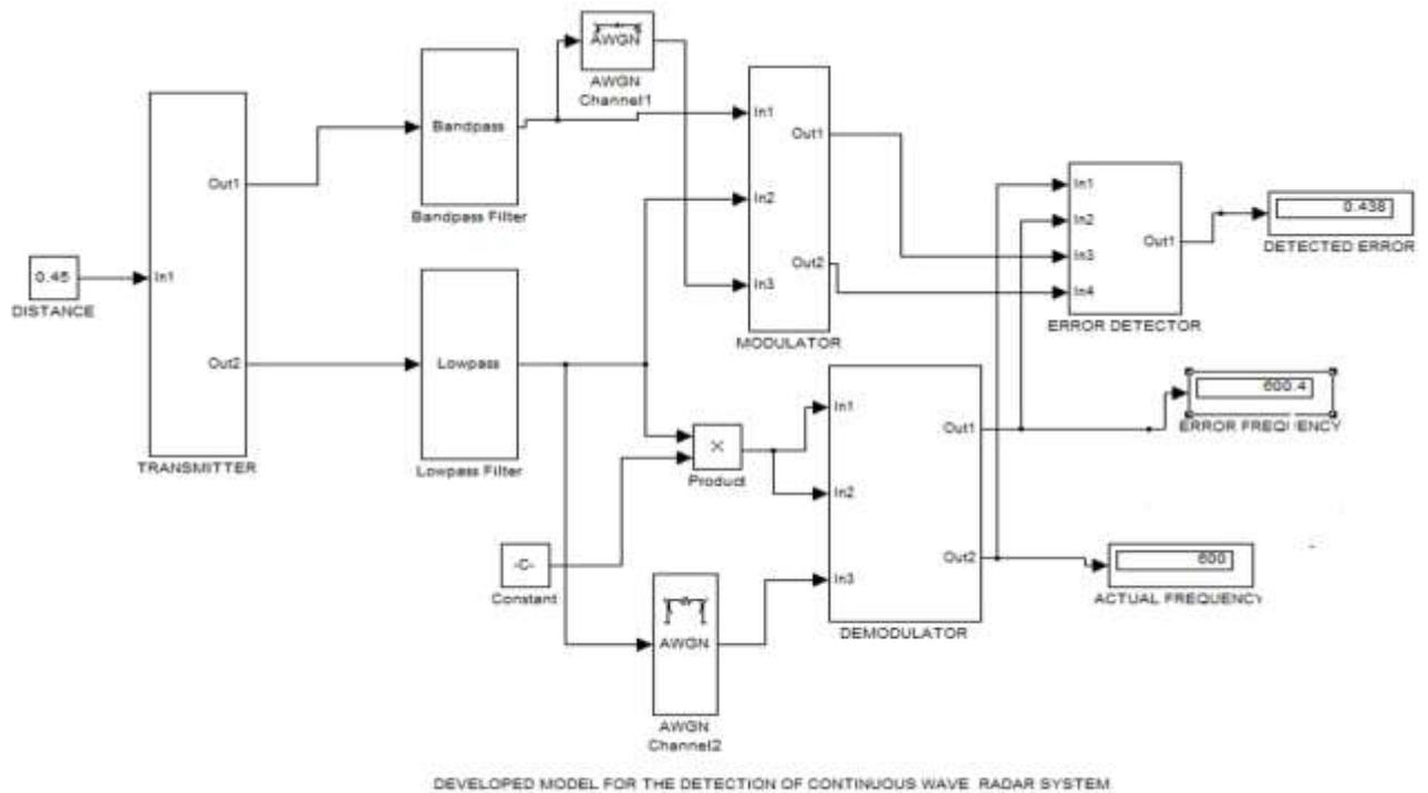
**Fig. 2:** Developed model for detection of Continuous Wave Radar System
