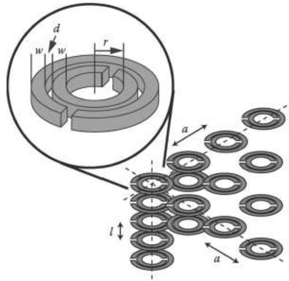
**Fig. 1:** Outline of the structure of basic optical metamaterials with an SRR used for the artificial control of magnetic permeability (Pendry et al., 1999)
