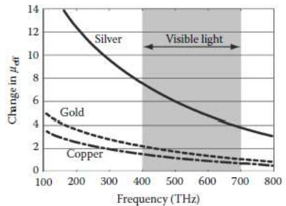
**Fig. 3:** The frequency dependence of change in  $\mu_{\text{eff}}$  of the SRRs consisting of silver, gold, and copper (Chon and Iniewski, 2013)
