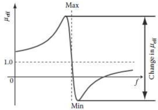
**Fig. 2:**  $\mu_{\text{eff}}$  changes in the positive and negative direction and takes the max  $\mu_{\text{eff}}$  and the min  $\mu_{\text{eff}}$  at the SRR resonant frequency (Chon and Iniewski, 2013)
