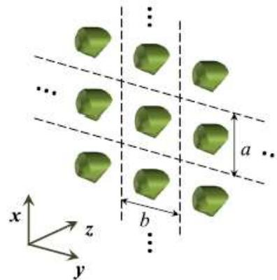
**Fig. 5:** A periodic infinite 2D metasurface (Zhao et al., 2014)
