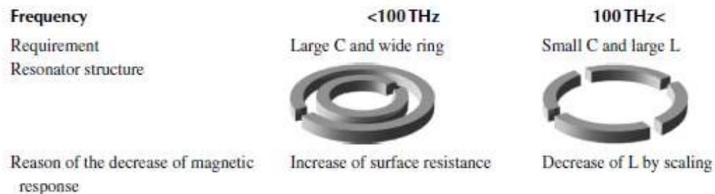
**Fig. 4:** The design approach of optical metamaterials in the optical frequency region revealing the active magnetic response below and above 100 THz (Chon and Iniewski, 2013)
