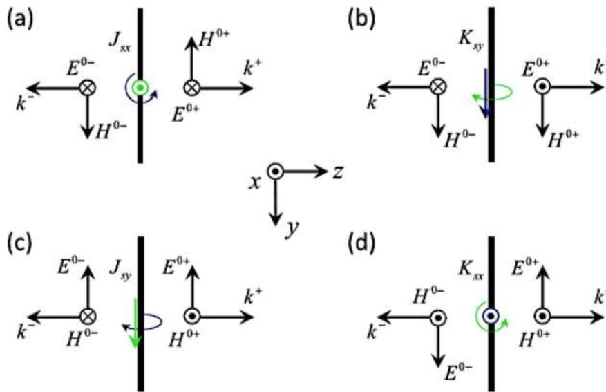
**Fig. 6:** Surface-induced currents and the radiated associated fields on the metasurface (Zhao et al., 2014)
