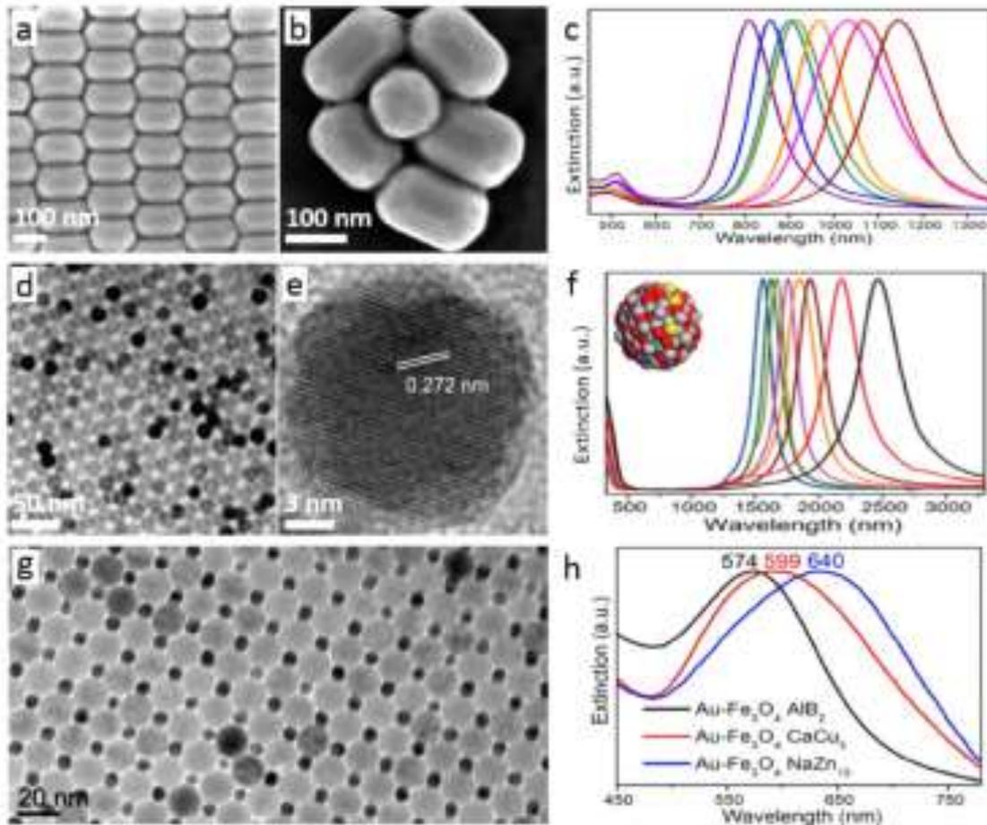
**Fig. 9:** (a) Low-resolution SEM image (b) high-resolution SEM image (c) the spectra display of Au nanorods. (d) Low-resolution TEM image (e) high-resolution TEM image (f) spectra display of CdO: F, in colloidal NPs. (g) TEM image (h) the spectra of  $Au-Fe_3O_4$  binary colloidal NP superlattices (Urbas et al., 2016)
