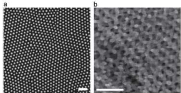
**Fig. 8:** SEM Images (a) hexagonal structure of Au dot array using thin-film deposition (b) a basic 3D Au network produced by electrodeposition template (Urbas et al., 2016).
