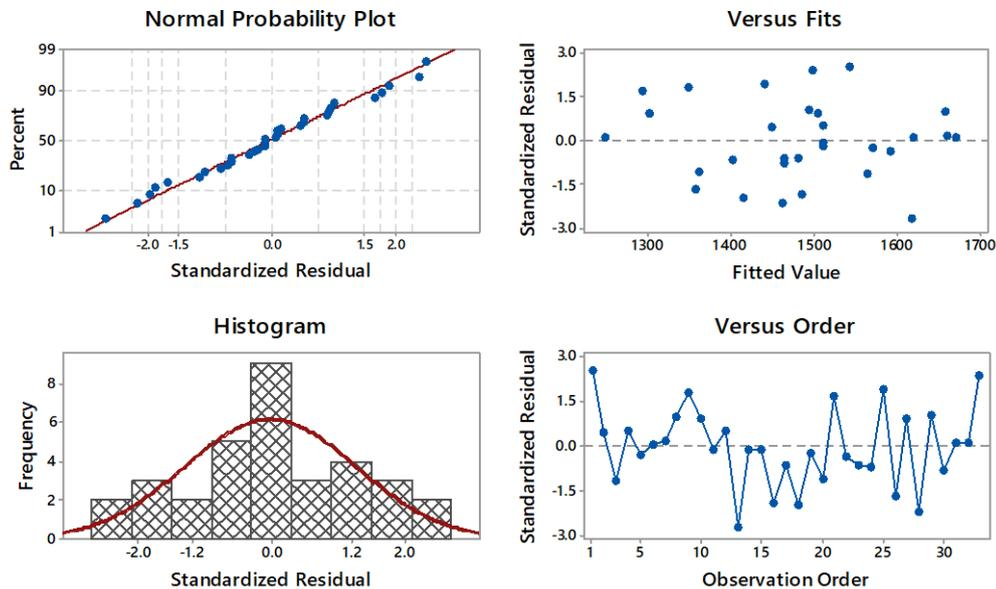
**Fig. 1:** Residual plots of the developed Ohiya clay's refractoriness function
