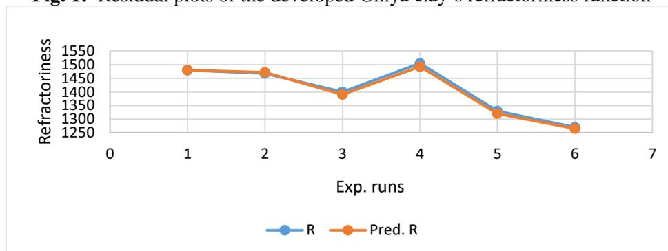
**Fig. 2:** Experimental confirmation of the developed Ohiya clay's refractoriness function
