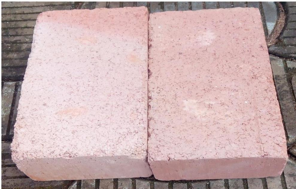
Fig. 4: Standard fireclay brick developed from Ohiya clay
