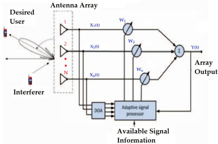
Fig. 1: Block diagram of smart antenna (Ashwim and Khyati, 2018)
