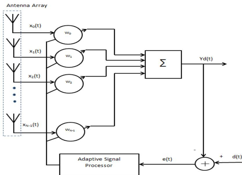
Fig. 3: Block diagram of adaptive antenna for MLMS algorithm
