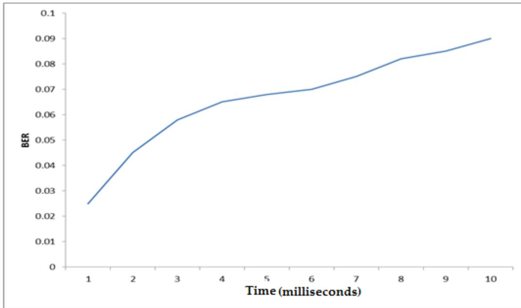
**Fig. 5:** Bit error rate performance analysis of simple adaptive antenna array using LMS algorithm
