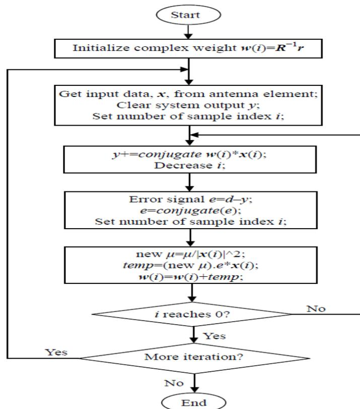
Fig. 2: Flow chart diagram for implementing LMS algorithm (Griffith, 1996)
