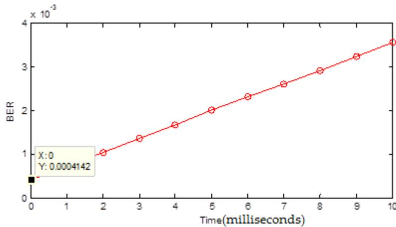
**Fig. 6:** Bit error rate graph when  $w_0=0.0001$  and  $\phi=0.0001$
