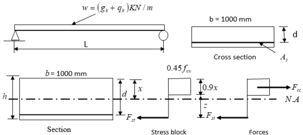
**Fig. 1:** A continuous one way reinforced concrete slab under uniform loading and assumed stress block
