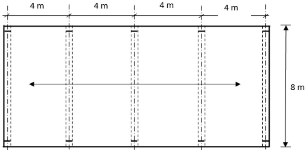
**Fig. 1:** A continuous one way reinforced concrete slab
