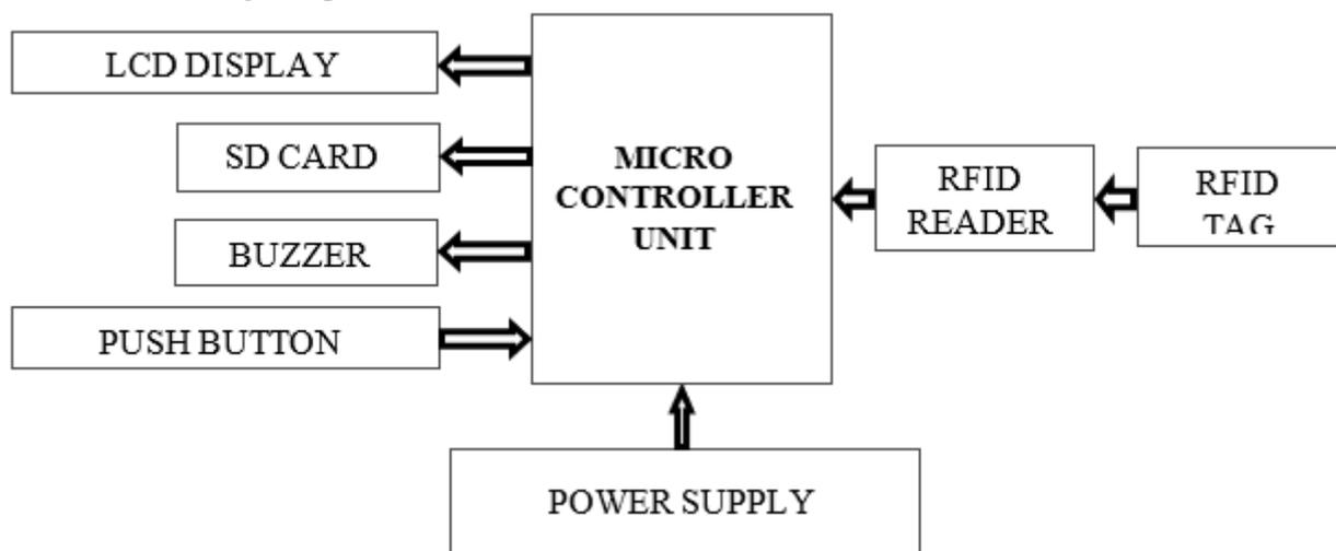
**Fig. 1:** Block diagram representation of the hardware circuitry.
