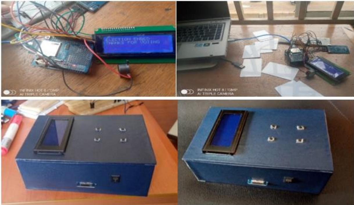
**Fig. 9:** Construction and packaging of the enhanced electronic voting machine
