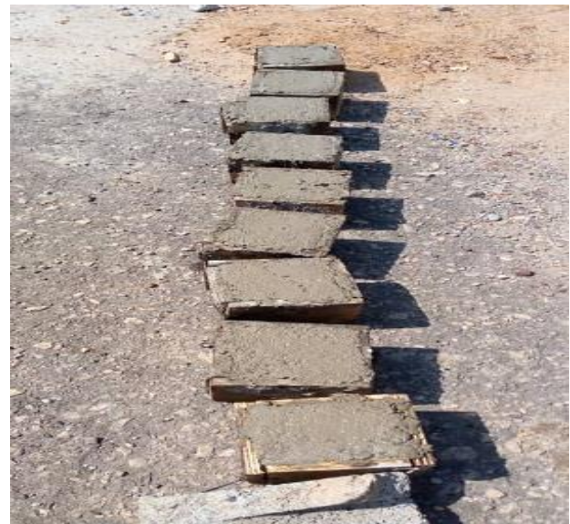
Fig. 1: Casted concrete cubes
