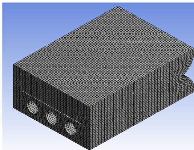
**Fig. 2:** Multi-block structured grids for the heat sink
