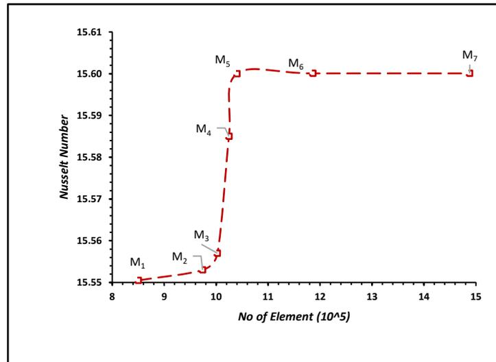
Fig. 3: Grid independence test
