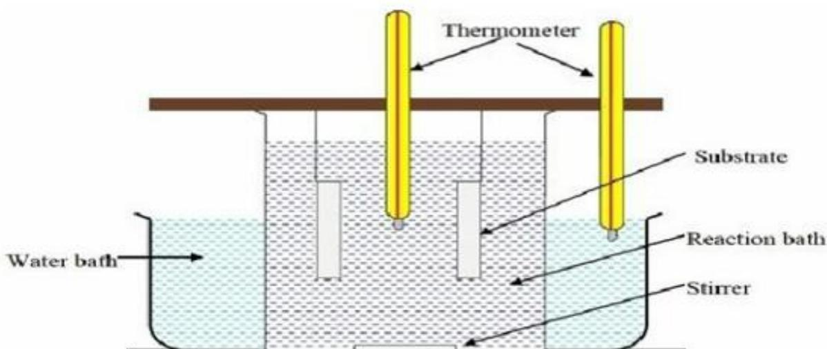
**Fig. 1:** Experimental set-up of Pb-Zn-S deposition (Zein and Alghoraibi, 2014)
