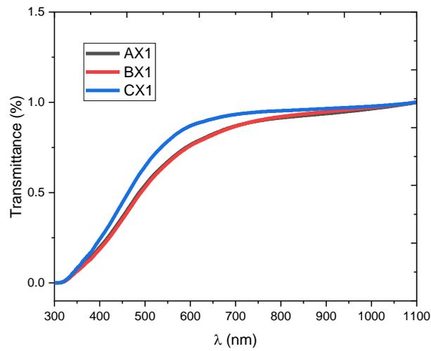
**Fig. 2:** Transmittance spectrum of PZS thin films
