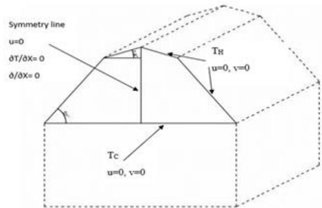
**Fig. 1:** 3D schematic diagram of gambrel roof type (Koca et al., 2007)
