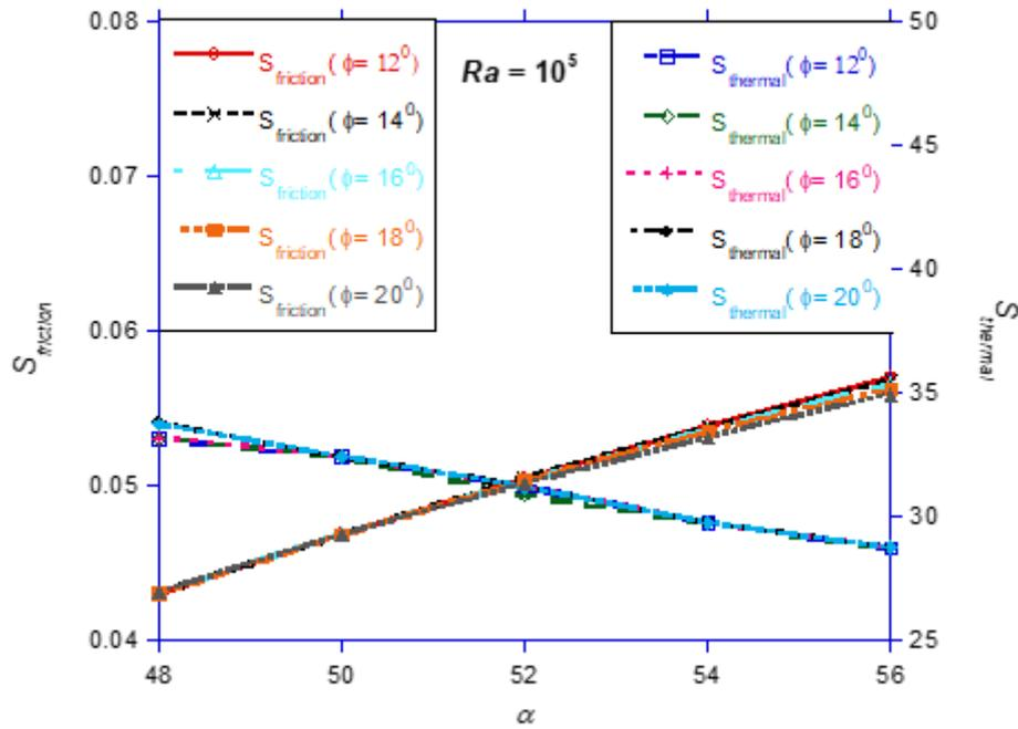
**Fig. 8:**  $\alpha$  against  $S_{thermal}$  and  $S_{friction}$  at different  $\phi$  at fixed  $Ra=10^5$
