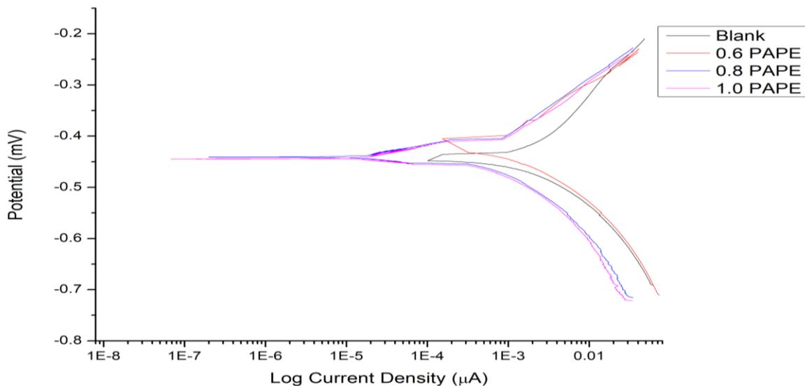
**Fig. 9:** Polarization curves of mild steel in 1M HCl with and without PAPE Inhibitor
