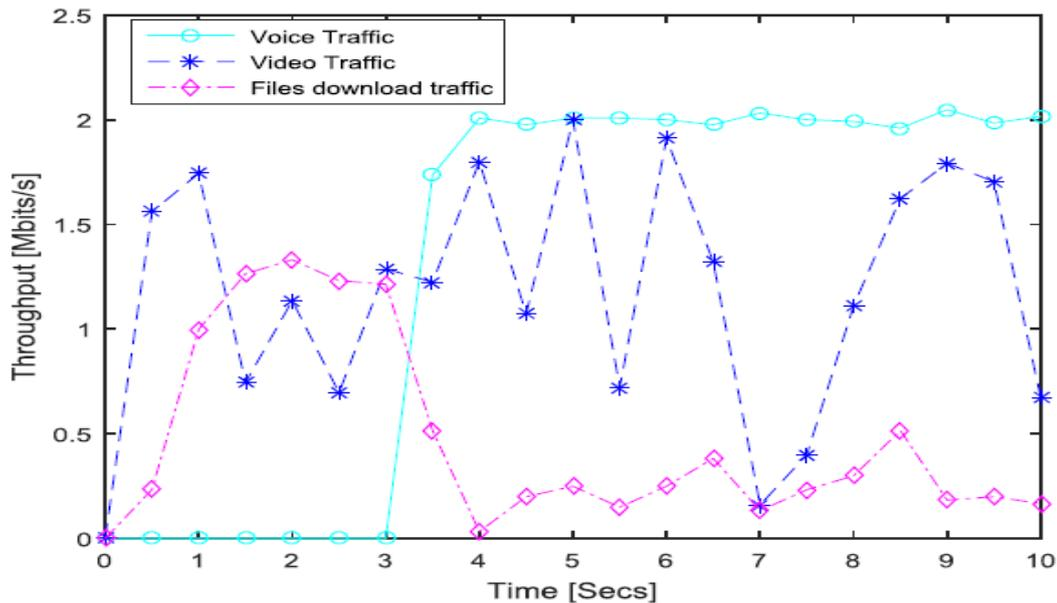
Fig. 5: Throughput in adaptive bandwidth allocation for voice traffic handover
