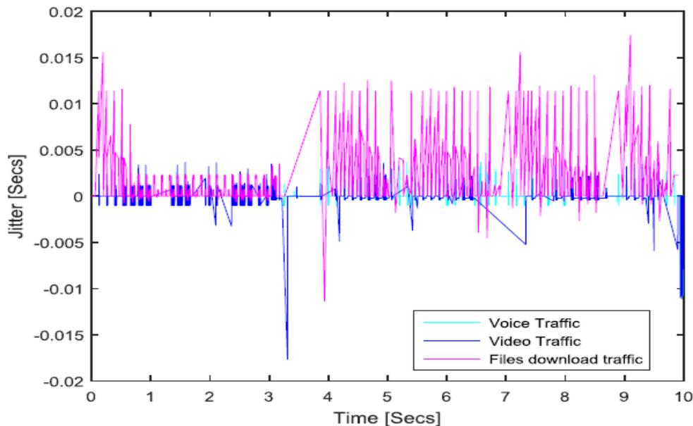
**Fig. 9:** Jitter in adaptive bandwidth allocation after voice traffic handover
