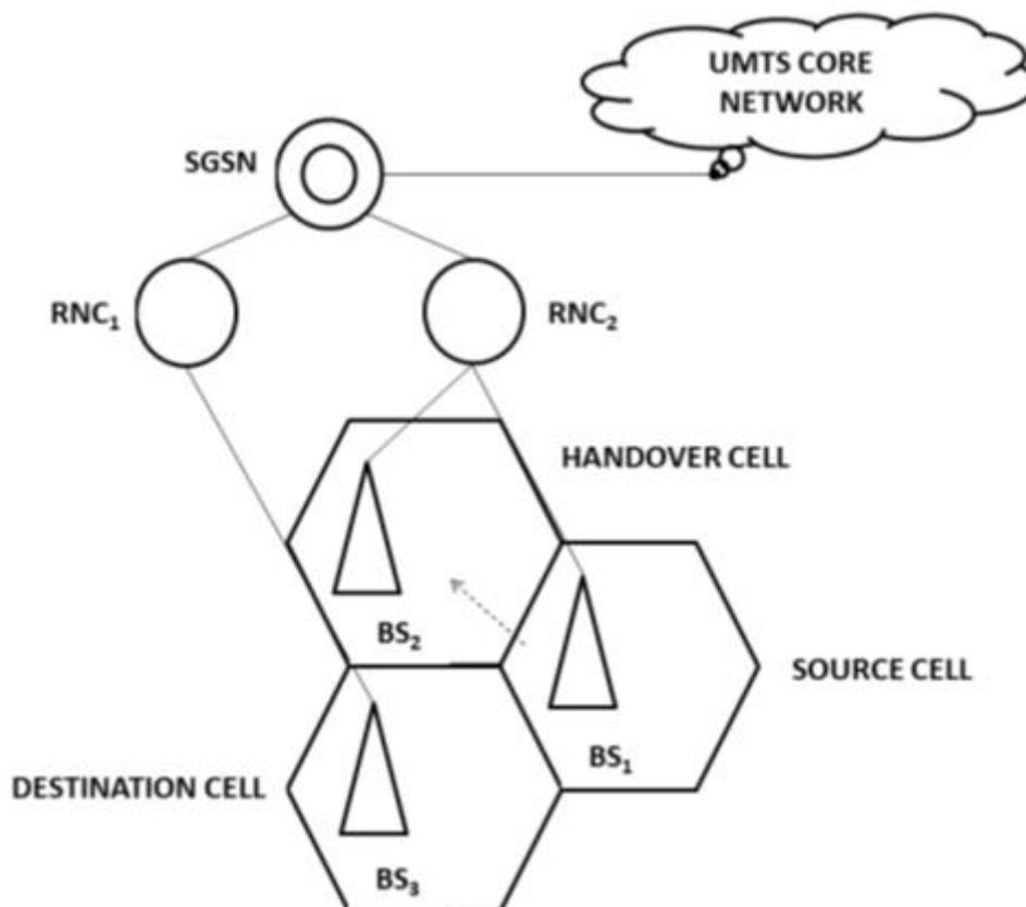
**Fig. 1:** Three cells arrangement in a Universal Mobile Telecommunication System (UMTS) network
