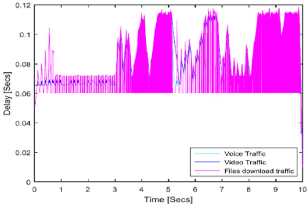
**Fig. 6:** Delay in conventional IP for voice traffic handover
