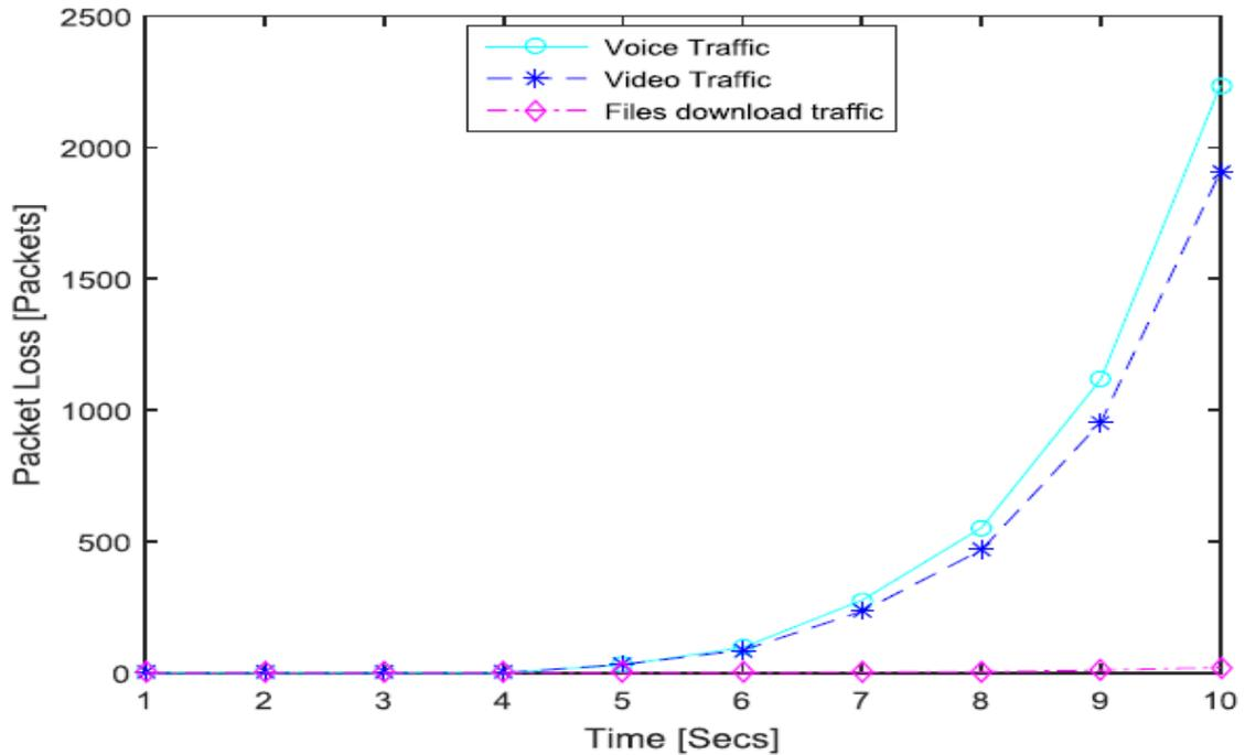
Fig. 2: Packet loss in conventional IP for voice traffic handover
