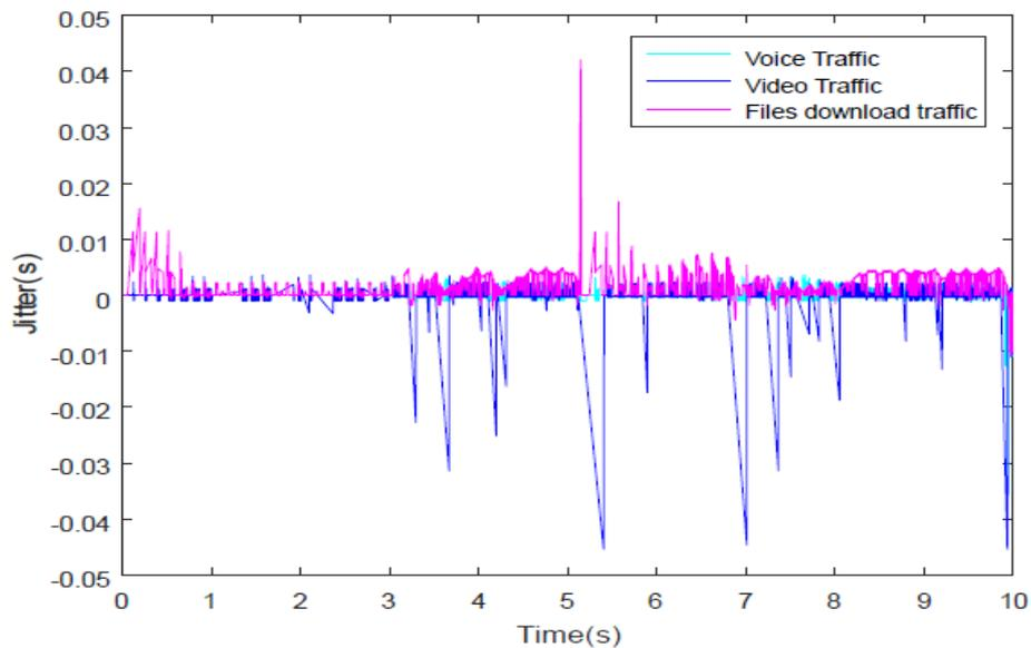
**Fig. 8:** Jitter in conventional IP for voice traffic handover
