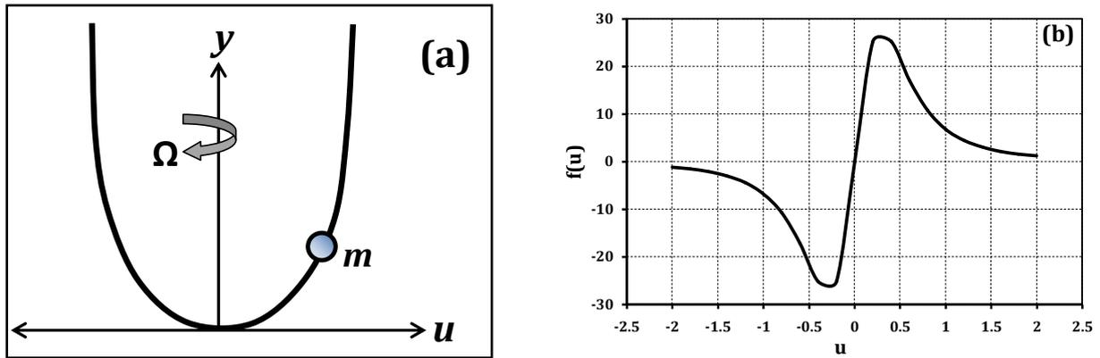
**Fig. 4:** (a) Schematic of particle on a rotating parabola (b) Restoring force when  $q = 1.0$ ;  $\Lambda = 10.0$  and  $A = 2.0$  (Source: Big-Alabo and Ossia, 2020).
