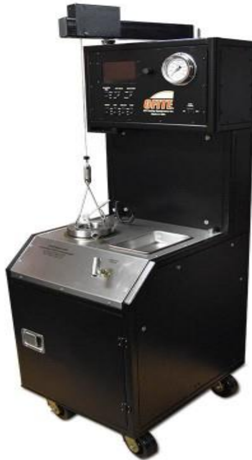
Fig. 1: Ofite HTHP Consistometer for thickening time test
