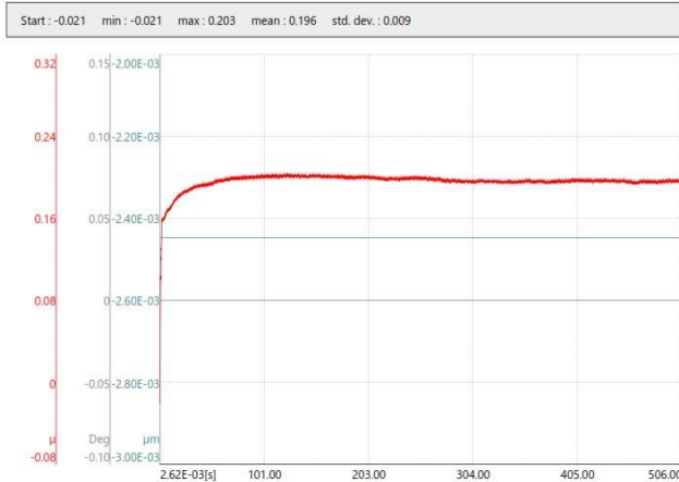
Fig. 12: Coefficient of friction of commercial brake pad (control 2)
