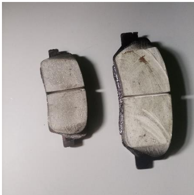
Fig. 15: The finished brake pad sample with 63 \mu m particle grain size
