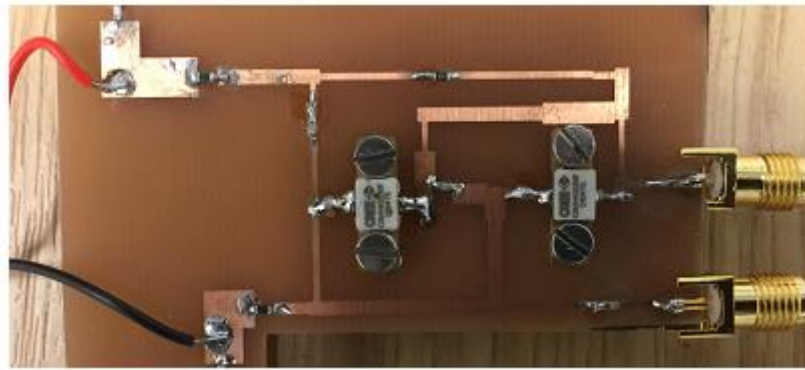
Fig. 5: PCB fabricated two-port negative reactance circuit
