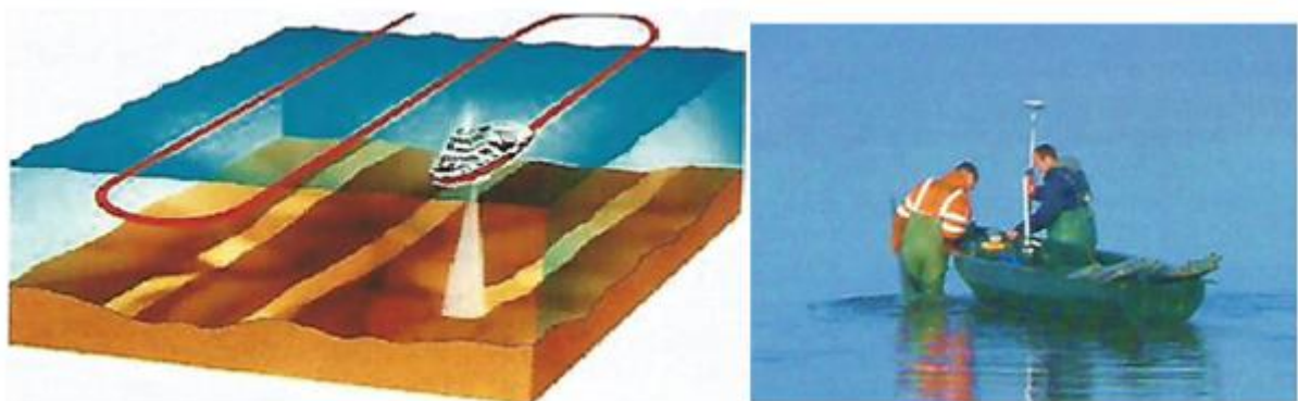
Fig. 3: Depth measurement with SB echo sounder and Position fixing with RTK GPS (Skilltrade, 2010)
